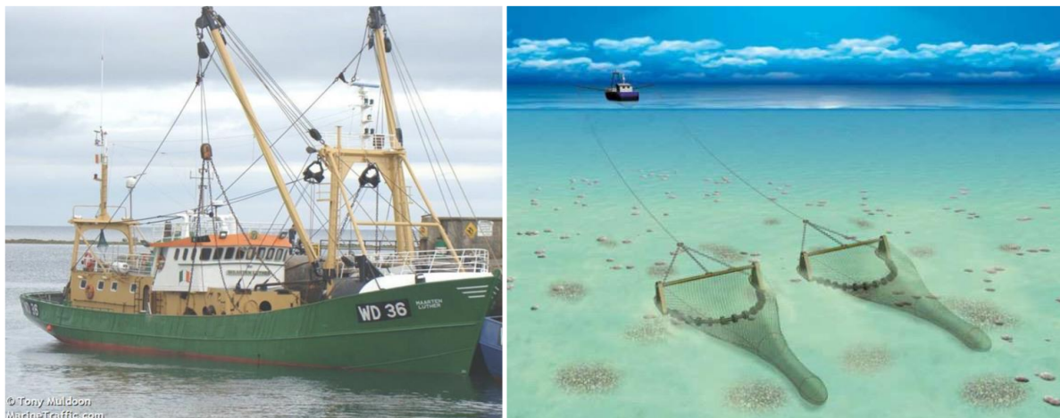
Plate 29 Typical beam trawling vessel and gear configuration (Source: Marine Traffic, 2020 and Seafish, 2015)
