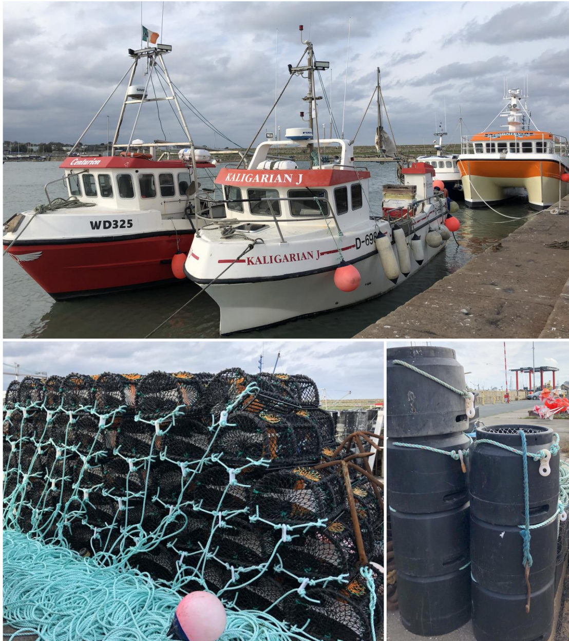
Plate 26 Typical potting vessels and gear at Dún Laoghaire Harbour; including creels used to target lobster and crab (bottom left) and plastic pots used to target whelk (bottom right) (Source: NiMa)
