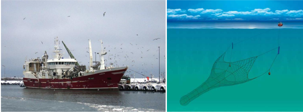
Plate 30 Typical pelagic trawling vessel and gear configuration (Source: NiMa; and Seafish, 2015)
