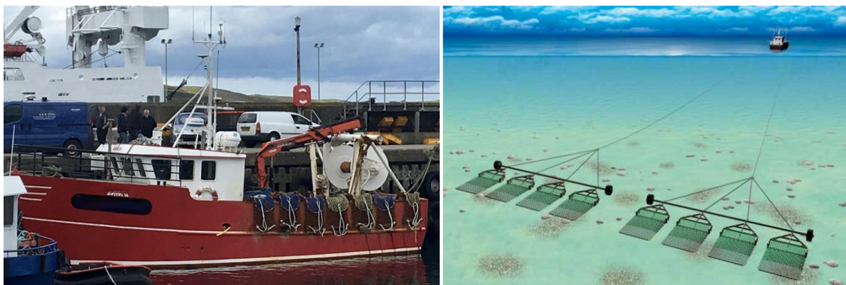
Plate 27 Typical scallop dredging vessel and gear configuration (Source: NiMa; and Seafish, 2015)
